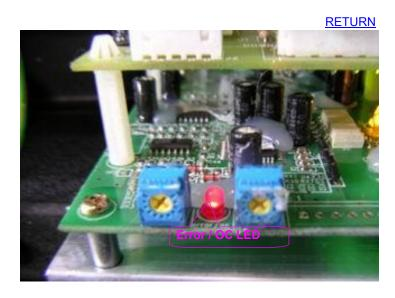
STEP 12 :Check upper board "start enable signal" is on or not (If D25 isn't on, change a new PCB)
